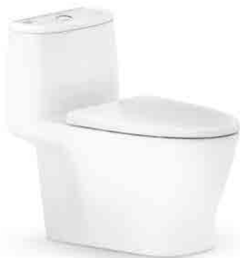
W372 x L720 x H695 Rimless with Double vortex, soft close seat cover 305mm, S-trap
